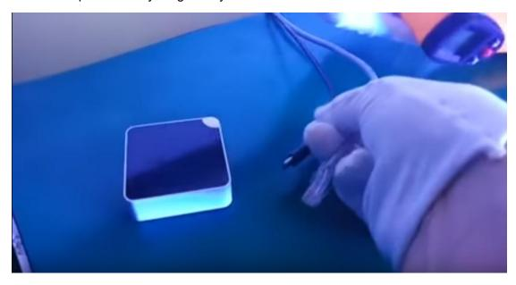
2. Rapidly plug the power supply in and out of the power receptacle four times. Your light should flash twice and remain on at 80% intensity.
