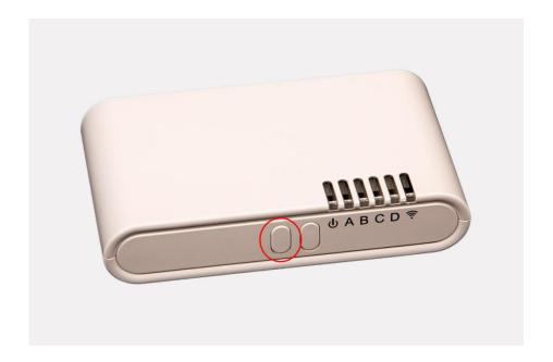
6. When the red LED (LED C) turns off, restart the gateway, then the upgrade process is Complete and you can press the reset button one time.
