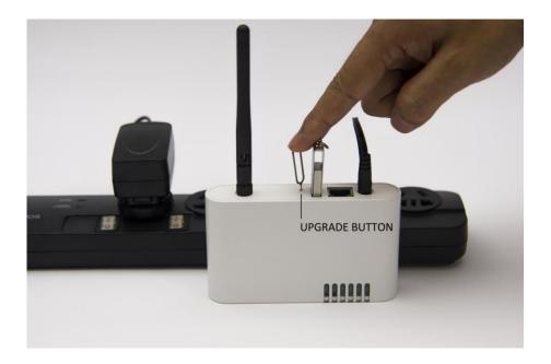
3. Press the upgrade button and while holding the button in, apply power to the gateway.
