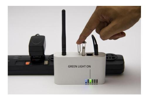
5. When all the 5 LEDs are on press the button marked in red circle one time. (Do not press the button till all LEDs light ON.) They come on and off quickly so you may not see them.
