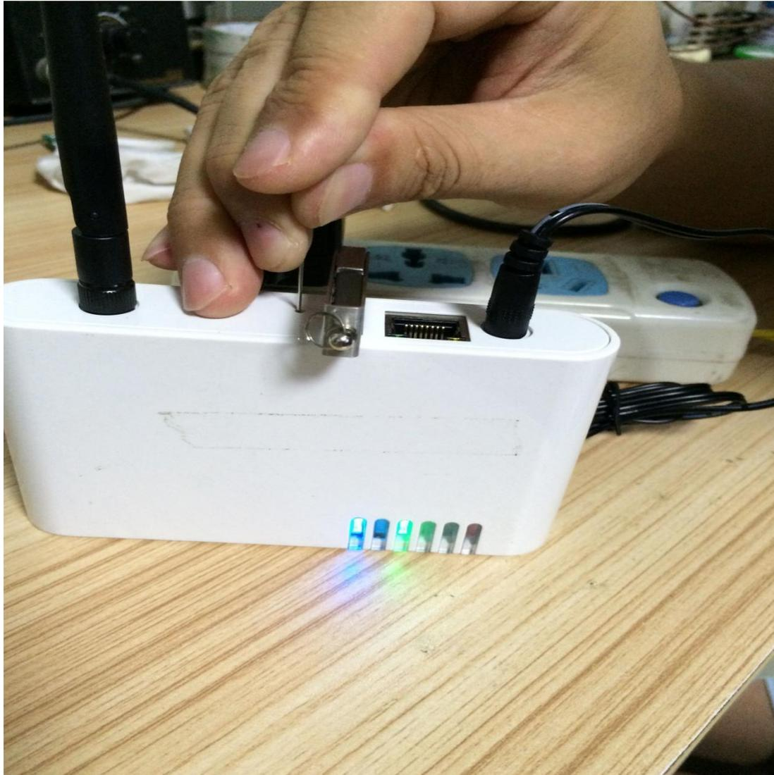
5. When all the 6 LEDs are on press the button marked in red circle one time. (Do not press the button till all leds light ON)
