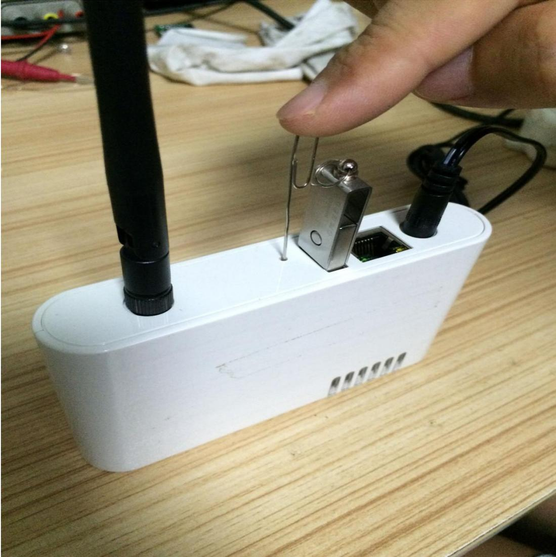
3. Press the upgrade button and then apply power to the gateway.
