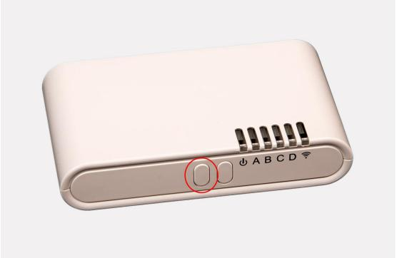
6. When the red LED (LED C) turns off, restart the gateway, then the upgrade process is complete.
