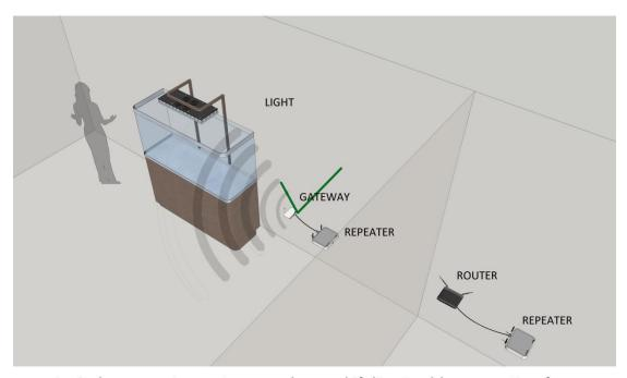
A wireless repeater system may be used if direct cable connection from the Gateway to the router is impractical in your installation
