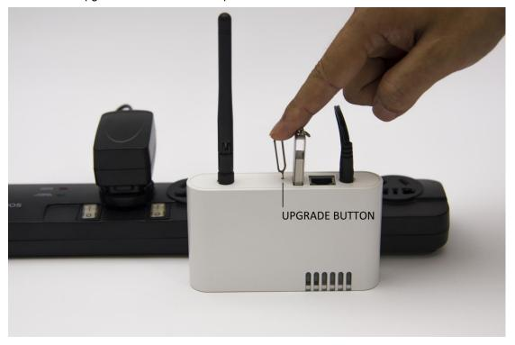
3. Press the upgrade button and then apply power to the gateway.
