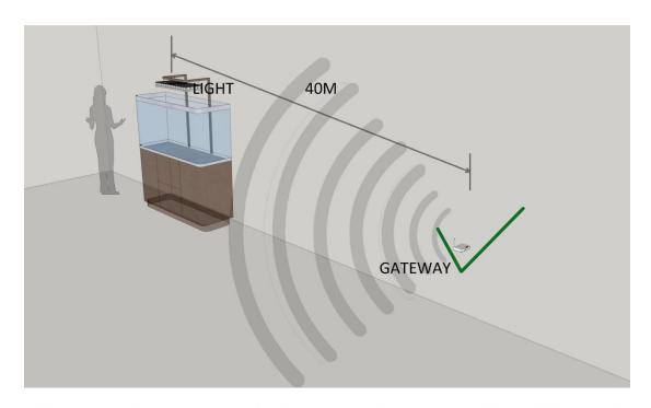
The distance from the light to the Gateway should not exceed 130 feet (40 meters).
