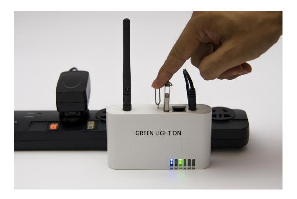
5. When all the 6 LEDs are on press the button marked in red circle one time. (Do not press the button till all leds light ON.)
