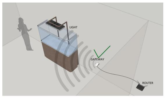
The WLAN router can be installed in any location in your home provided the Ethernet cable is connected to the Gateway.
