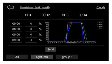
The above screen shot for this channel explains what this channel does very well. Here we have all channels at 100% intensity but for an increased time span at 100%. This channel provides all the PAR/PUR the Atlantik V4 / Atlantik Compact V4 can deliver. This channel is not recommended for fragging.
