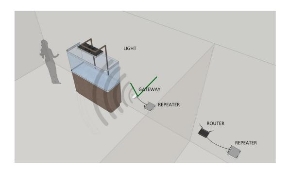
5.A wireless repeater system may be used if direct cable connection from the Gateway to the router is impractical in your installation.
