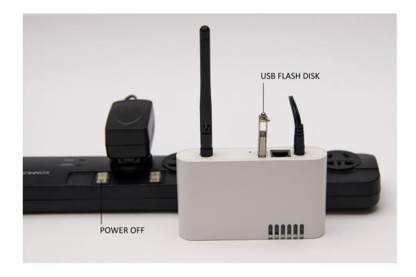
STEP 1 Plug in USB Flash Disk after you have downloaded the upgrade software.
