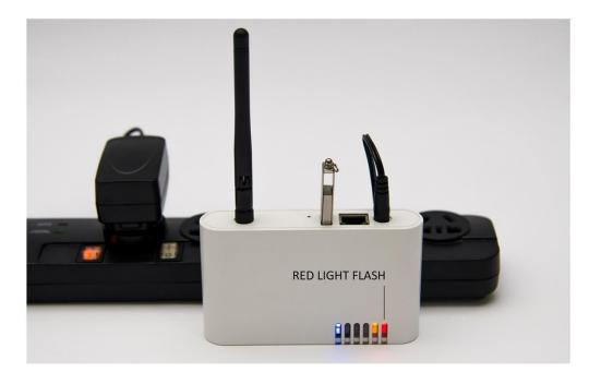
**STEP 5** When the red light flashes, the upgrade process complete.
