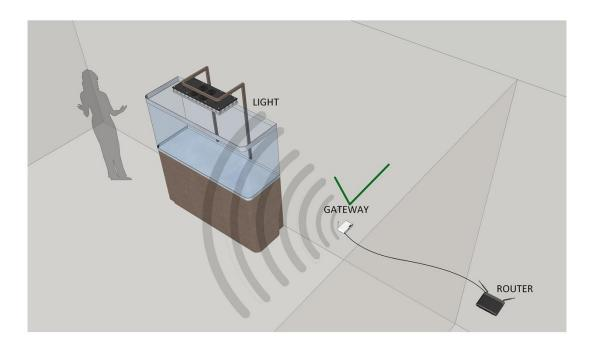
4. The WLAN router can be installed in any location in your home provided the Ethernet cable is connected to the Gateway.
