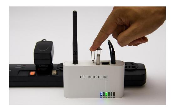
**STEP 4** The green light will flash. Release the upgrade button when the green light stops flashing and remains on.
