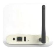
2. Connect the Gateway to your router using a standard Ethernet cable.
