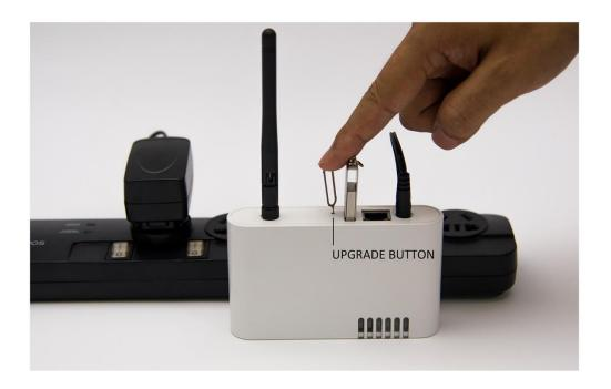
STEP 2 Press the upgrade button with a paper clip or other tool that can enter the hole.
