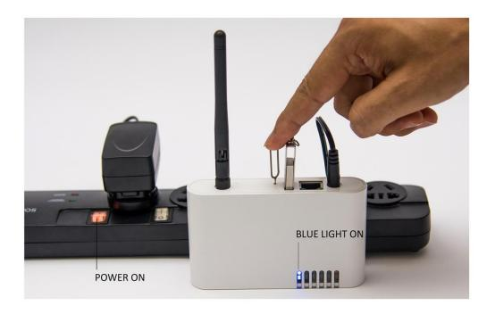
**STEP 3** Press the upgrade button and then apply power to the gateway.
