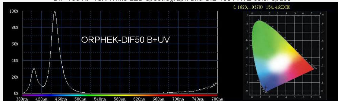
DIF 50 / 100 BLUE UV LED spectrograph and CIE 1931 XYZ color space
